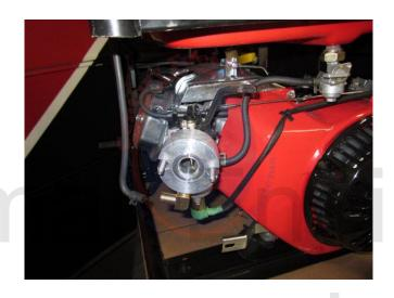
Push the Adaptor, with the venturi inside, onto the stud extenders. Make sure the brass fitting is attached to the bottom.
