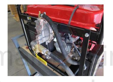
Clamp vapor hose between the regulator and adaptor.
